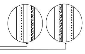
Pre-tapped 12-24 threaded holes on one side and square rack holes on the other. According to the installation requirements choose threaded or square at front.
